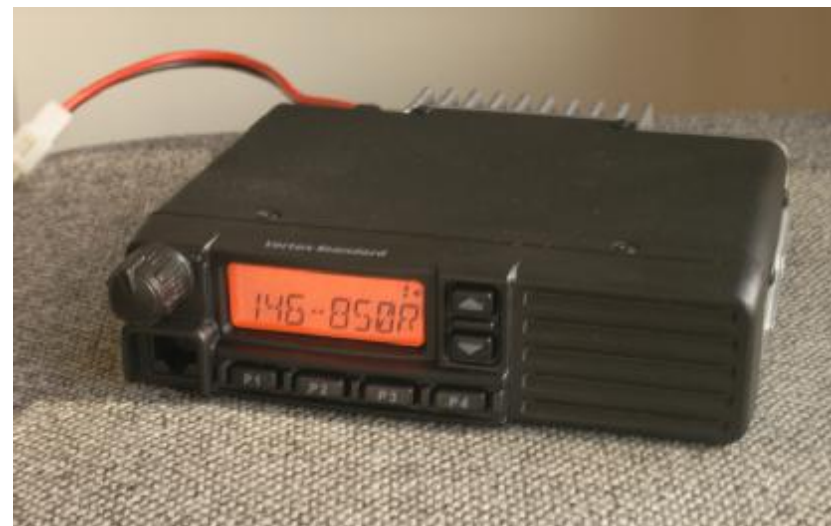
Fig.2 VERTEX radio for channels in the band 136—170 MHz
