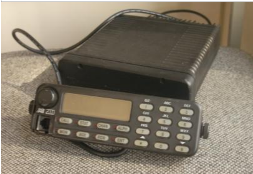
Fig.1 TAIT radio for channels in the band 70—85 MHz
