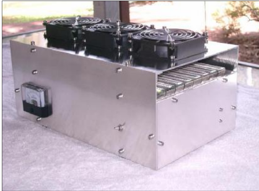
Fig.3 Ericson cell phone transmitter for 2301 MHz. Chassis and cooling system by Trevor VK4AFL
