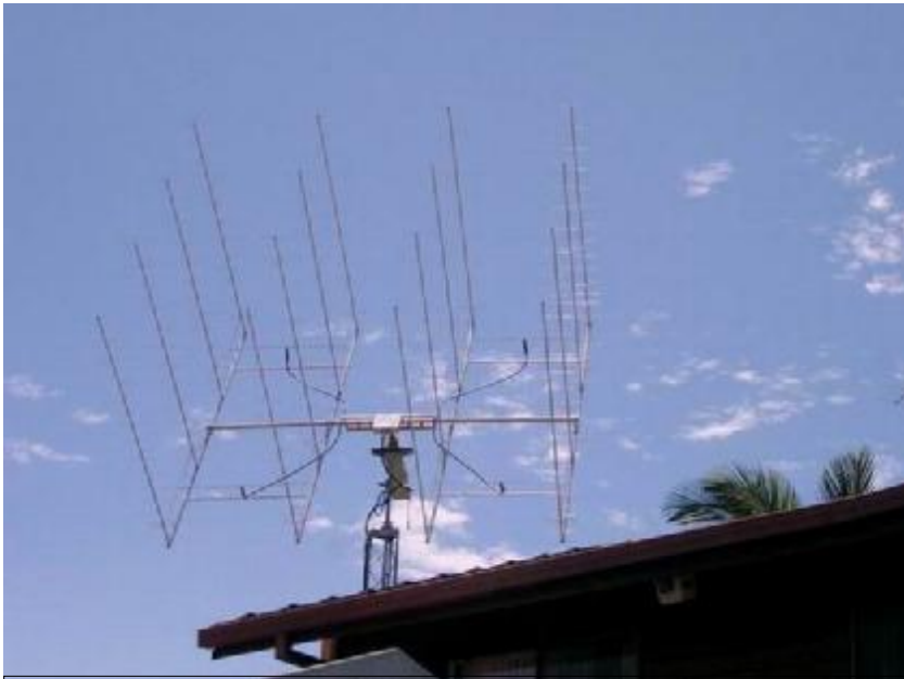
Fig.1 The VK4AFL antenna for 432 MHz EME operation It comprises 16 x 15 element linear Yagis mounted on an AZ-EI rotator which also rotates about its bore axis for polarity control.
