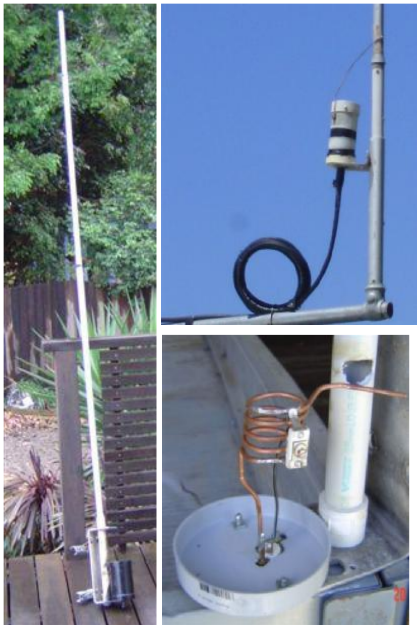
Six metre half-wave vertical antenna Clockwise from left: Complete antenna, coil assembly installed for repeater site, parallel coil and capacitor .
