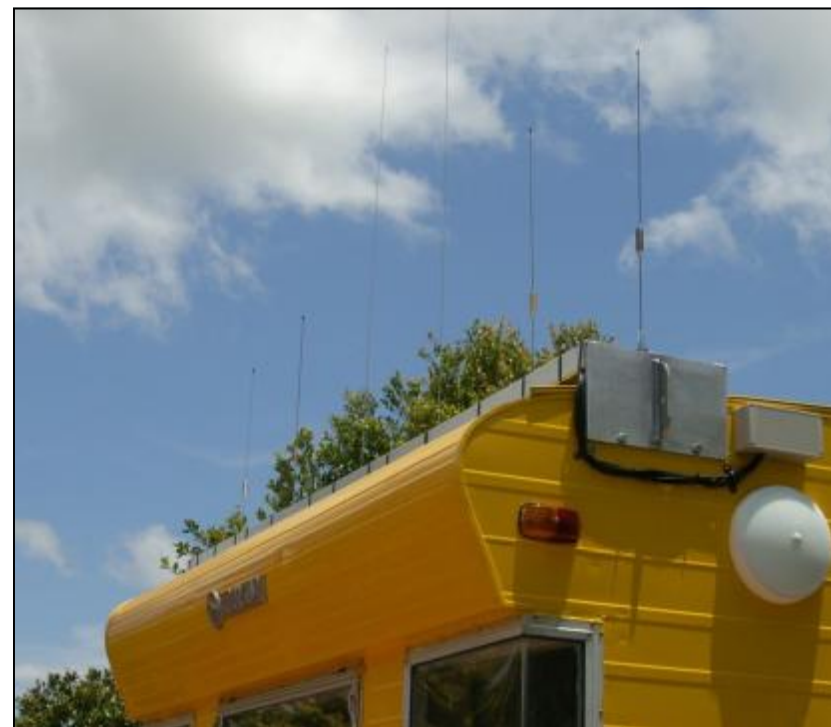
WICEN caravan antennas Pictured are six of the many antennas for 6 m, 2 m and 70 cm. Each will be tuned to its band of frequencies. For HF a 7 m vertical antenna will be mounted on the front lower to provide communications on 40 m and 5 MHz.
