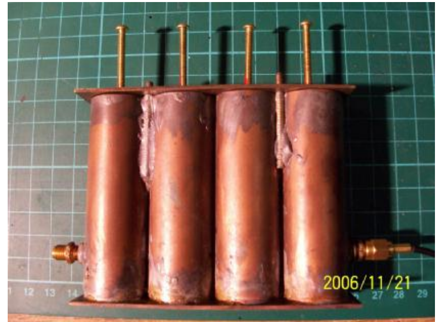
Fig.3 Final assembly of cavities with SMA connectors
