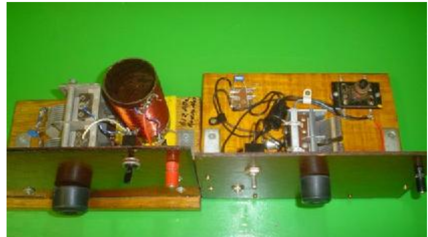
Two basic un-powered crystal sets built by Rod VK4MRC
