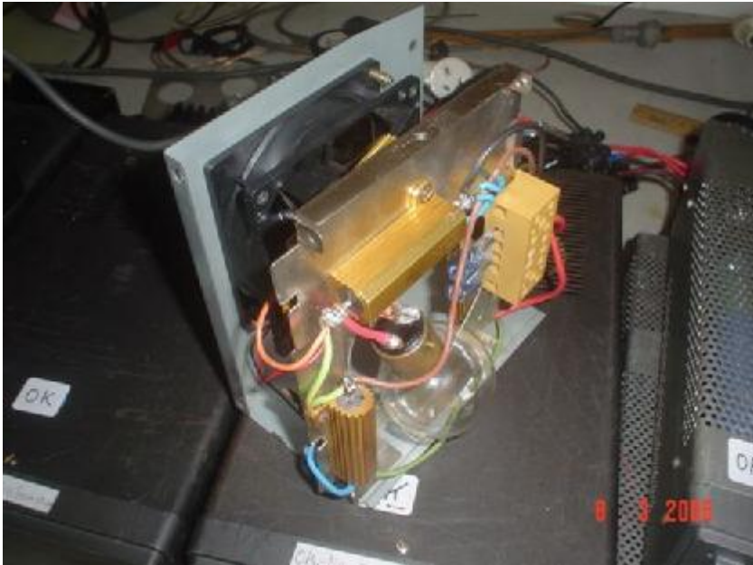
Fig.1 16 A resistive load for Kenwood power supplies
