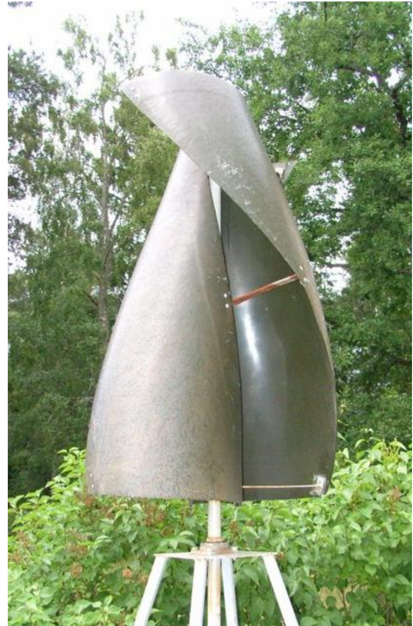
The bi-conical rotor of the wind-powered generator invented by the Fins
