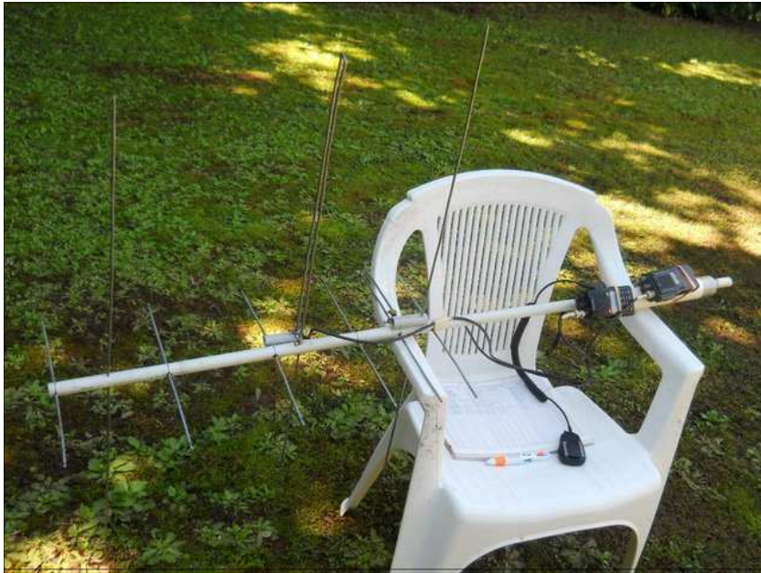
Fig.1 Harvey VK4AHW satellite radio and tracking system 144 Mhz uplink—435 MHZ downlink
