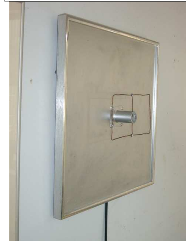
Fig. 2 Square quad pair with centre freq 852 MHz Picture frame has 36 mm square AL sheet
